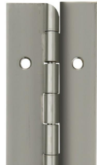
Satin Stainless Steel Grade 304 Continuous Ball Bearing Hinge, 75mm x 2000mm x 2.5mm. 12mm diameter knuckle to suit up to 200kg maximum weight.
